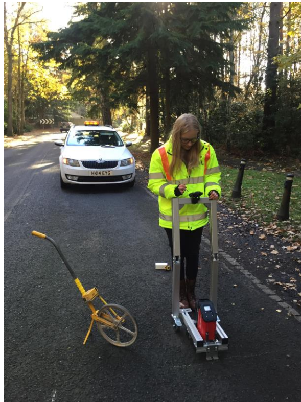
Figure 31: Researcher using the mobile trolley to capture spectra
